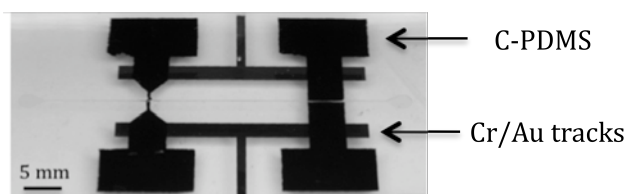
Figure 1. Photograph of the microfluidic device with a 200 \mu\text{m} wide channel and C-PDMS electrodes. Gold tracks providing ohmic contact are visible.
