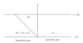
FIGURE 1. The interface states  $\mathbf{U}^* = (u^*, v^*)$  are linked to  $(u_L, v_L)$  by the 1-wave of speed  $-a/\varepsilon$ , and to  $v_R$  by imposing the continuity of the numerical flux of v.
