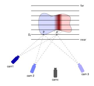
Fig. 1. Plane-sweep : geometric configuration
