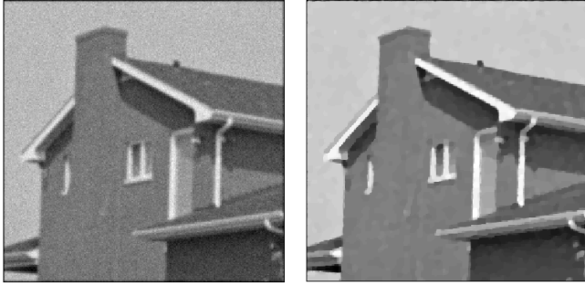
Fig. 1. Noisy blurred image with Gaussian blur, \alpha = 0.1 and \beta = 50 , SNR=22 dB, MSSIM=0.525 (left) and deblurred image (right) with the proposed algorithm, SNR=27.1 dB, MSSIM=0.835.
