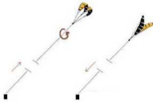
Fig. 4. Rotokite operation principal [50].
