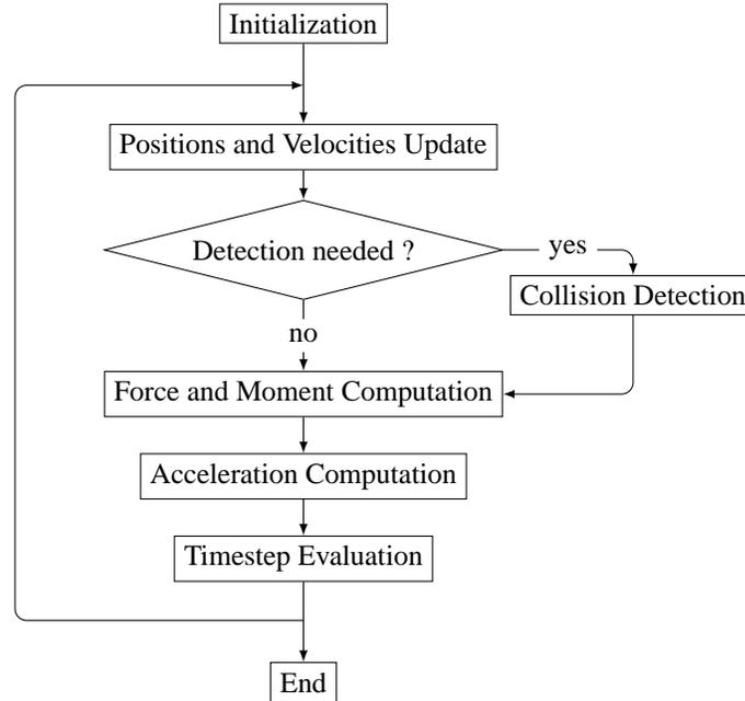
Figure 1: Global simulation integration scheme.
