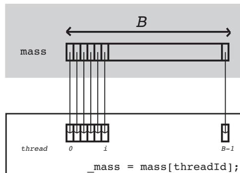
Figure 4: Illustration of a data load from global memory (grey zone) to thread registers. Every thread within a warp loads its value and this is done in a single coalesced memory transfer.
