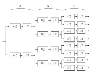
Figure 3. Analysis filter bank for a 3D Discrete Wavelet Transform.
