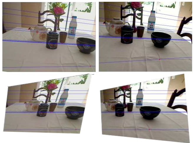
Fig. 2: Rectified image pair using Hartley [3] : the epipolar lines are horizontal and aligned from an image to the other. The rectified images are suited for computer vision processing, but not for stereoscopic rendering.
