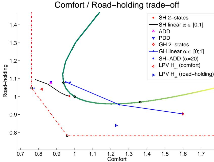
Figure 12: Normalized performance criteria trade-off for the presented control algorithms, compared to the passive suspension system, with damping value  $c \in [c_{min}; c_{max}]$  (solid line with varying color), optimal comfort and road-holding bounds (red dash dotted).
