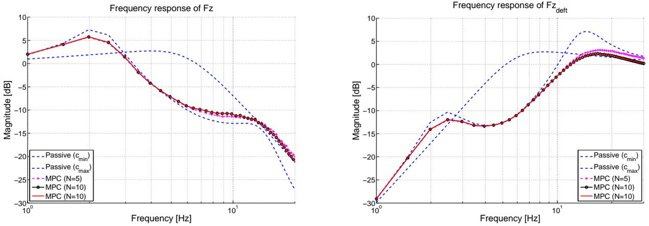
Figure 5: Results of the road-holding-oriented optimisation (*i.e.* cost function  $J_{rh}$ ) with varying prediction horizon  $N$ . Left: approximate FR from the road vertical acceleration to the body vertical acceleration. Right: approximate FR from the road profile to the tire deflection.
