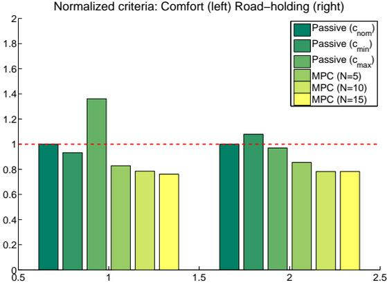
Figure 6: Performance criteria (normalized with respect to performance obtained with nominal damping  $c_0 = c_{nom}$ ). Optimal performance with respect to the prediction horizon  $N$ , compared to the passive settings. Left: comfort optimisation ( $i = c$ ). Right: road-holding optimisation ( $i = rh$ ).
