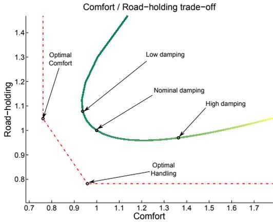
Figure 7: Comfort-road-holding trade-off ( $\{J_z, J_{z_{def_t}}\}$ ) for a passive suspension, with damping value  $c \in [c_{min} c_{max}]$  (solid line with varying color) and optimal comfort / road-holding bounds, with  $\alpha \in [0 1]$  (red dash dotted).
