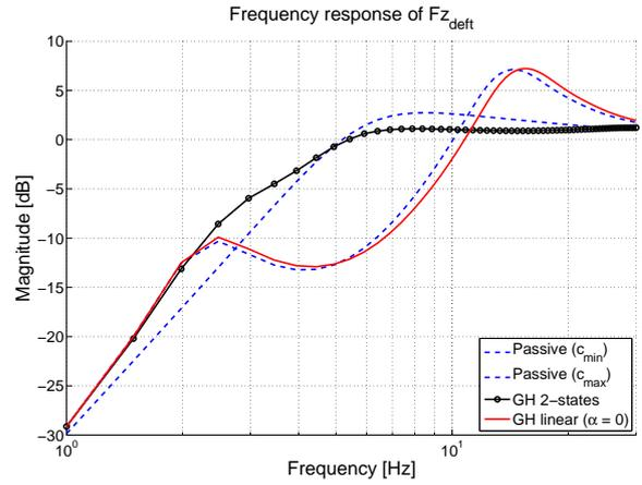
Figure 9: Road-holding oriented control law frequency response  $F_z$  (left) and  $F_{z_{def}}$  (right).
