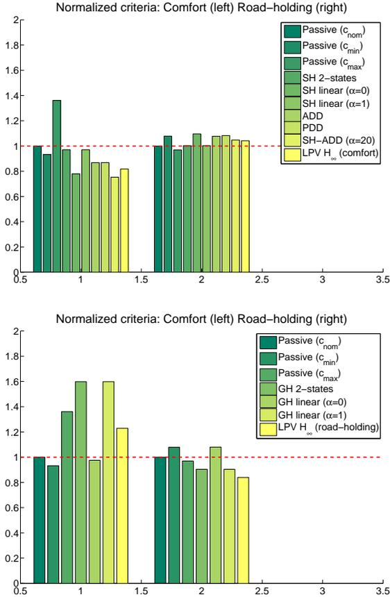
Figure 11: Normalized performance criteria comparison for different comfort (resp. road-holding) oriented control strategies. Comfort criteria - when cost function is  $J_c$  (left histogram set) and Road-Holding criteria - when cost function is  $J_{rh}$  (right histogram set).
