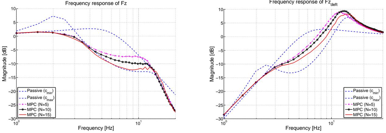
Figure 4: Results of the comfort-oriented optimisation (*i.e.* cost function  $J_c$ ) with varying prediction horizon  $N$ . Left: approximate FR from the road vertical acceleration to the body vertical acceleration. Right: approximate FR from the road profile to the tire deflection.
