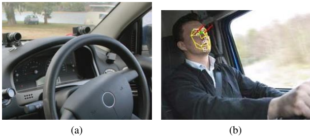
Fig. 4: The eye-tracker Facelab
