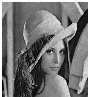
Figure 7: SigShrink denoising of the ‘Lena’ image corrupted by speckle noise. The SWT with four resolution levels and the Haar filters are used. The noise standard deviation is estimated by the MAD normalized by the constant 0.6745 (see [13]).
