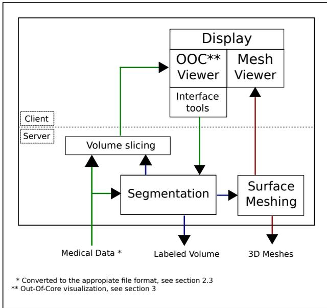
**Figure 6:** Block diagram of the segmentation application
