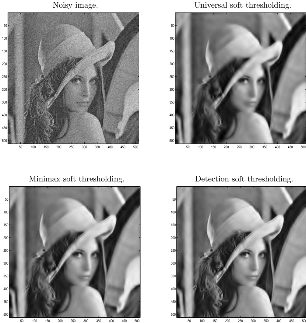
Figure 6: Noisy ‘Lena’ image and denoised images by soft thresholding with detection, minimax and universal thresholds. The noise standard deviation is \sigma = 25 . The wavelet transform used is a discrete stationary wavelet transform based on the ‘sym8’ wavelet. The thresholding is applied to the detail coefficients at decomposition levels j = 1, 2, 3, 4 .
