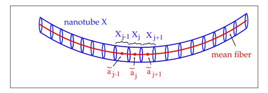
Figure 6: Mean fiber  $\tilde{a}_j$  of a nanotube
