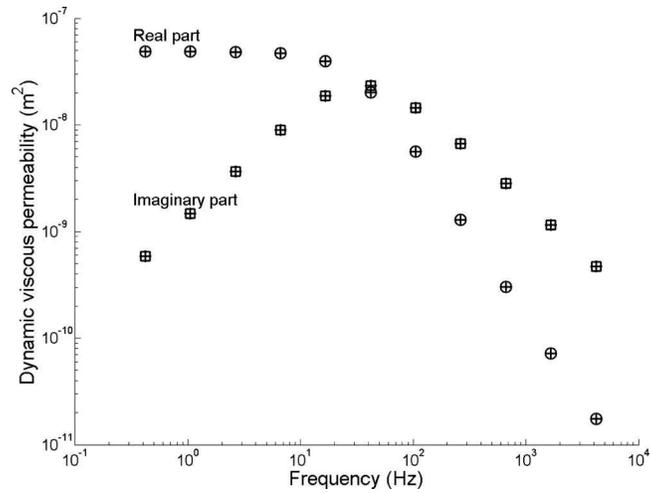
Fig. 2. Dynamic viscous permeability of a hexagonal lattice of solid cylinders: There is an almost perfect superposition of the permeability values computed from any orthogonal line pairs perpendicular to the sixfold axis of symmetry, suggesting that this property might be used for a convergence check.
