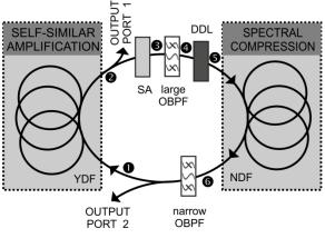
Fig. 1: Schematic of the laser.
