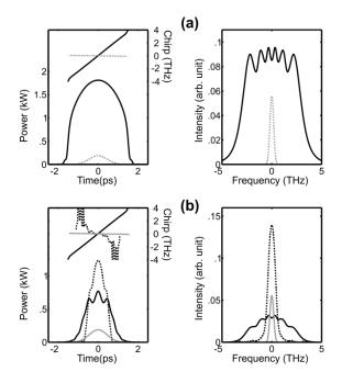
**Fig. 4:** Temporal intensity and chirp profiles (left) and spectral intensity profiles (right) of the pulse at (a) the entrance (location ① in Fig. 1; dotted curves) and the exit (location ② in Fig. 1; solid curves) of the gain fibre, and (b) the entrance of the passive fibre (location ③ in Fig. 1; solid black curves), the end of the passive fibre (location ③ in Fig. 1; dotted black curves), and after the narrow spectral filter and output coupler (location ① in Fig.1; solid gray curves).
