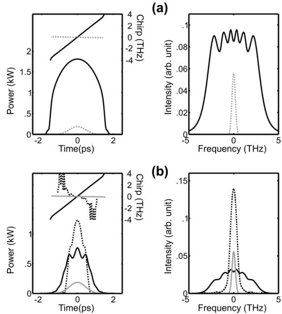
**Fig. 4:** Temporal intensity and chirp profiles (left) and spectral intensity profiles (right) of the pulse at (a) the entrance ( location ❶ in Fig. 1; dotted curves) and the exit (location ❷ in Fig. 1; solid curves) of the gain fibre, and (b) the entrance of the passive fibre (location ❸ in Fig. 1; solid black curves), the end of the passive fibre (location ❹ in Fig. 1; dotted black curves), and after the narrow spectral filter and output coupler (location ❶ in Fig.1; solid gray curves).
