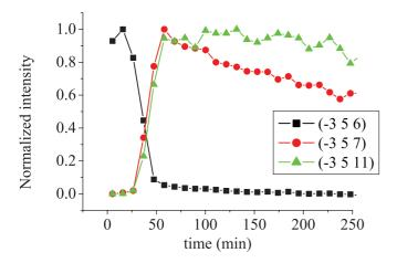
FIG. 9. (Color online) Normalized intensity variation of the (-356), (-357), and (-3511) diffraction peaks as a function of time during the isothermal relaxation at 40 K. The indexing of the three diffraction peaks refers to the triple C-centered cell of state  $\Pi^{\text{Relax}}$ .
