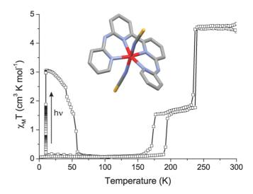
FIG. 1. (Color online) Molecular structure of **1**, and temperature dependence of the  $\chi_M T$  product, showing the two-step thermal spin transition, the photoexcitation, and the subsequent relaxation (Ref. 41).
