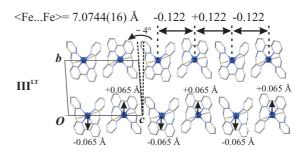
FIG. 3. (Color online) Section of the crystal packing in the (bc) plane indicating the displacement of the Fe<sup>II</sup> atoms along the **b** direction from the regular y = 0 position, and Fe...Fe separation distances along the **c** direction with respect to the average Fe...Fe distance. HS Fe<sup>II</sup> centers are shown in red, LS Fe<sup>II</sup> centers in blue. Hydrogen atoms have been omitted for clarity.
