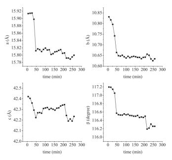
FIG. 7. Evolution of the unit cell parameters during the isothermal relaxation at 40 K from the photoinduced metastable state  $I^{LIESST2}$ . The  ${\bf c}$  axes for states  $I^{LIESST2}$  and III were multiplied by a factor of 3 for ease of comparison with state  $I^{Relax}$ .
