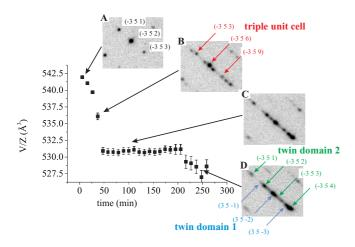
FIG. 6. (Color online) Evolution of the unit cell volume per formula unit (V/Z) during the isothermal relaxation at 40 K from the photoinduced metastable state I<sup>LIESST2</sup>, and selected region of the diffraction pattern centered on the [-3.51] row.
