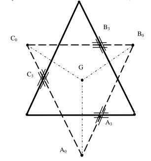
Fig. 1 The 3-PRP planar parallel robot
