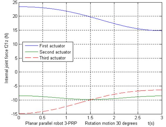
Fig. 8 Internal joint forces  $f_{21z}^A, f_{21z}^B, f_{21z}^C$
