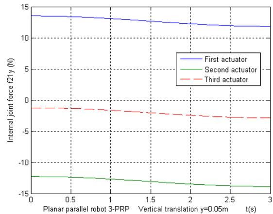
Fig. 4 Internal joint forces  $f_{21y}^A, f_{21y}^B, f_{21y}^C$
