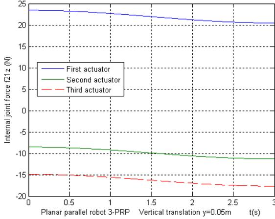
Fig. 5 Internal joint forces  $f_{21z}^A, f_{21z}^B, f_{21z}^C$
