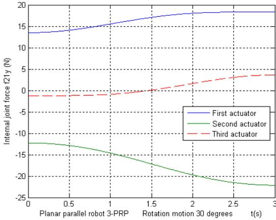
Fig. 7 Internal joint forces  $f_{21y}^A, f_{21y}^B, f_{21y}^C$
