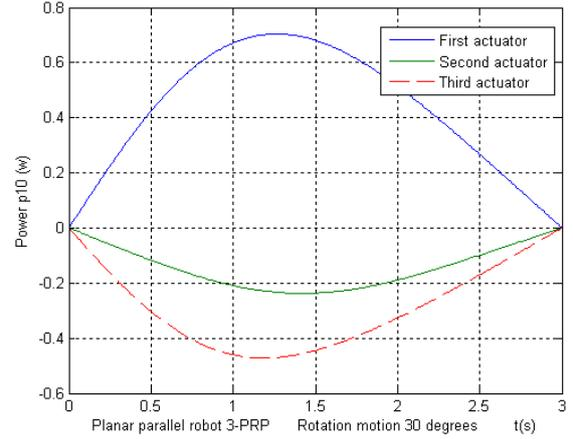
Fig. 6 Powers  $p_{10}^A, p_{10}^B, p_{10}^C$  of three actuators
