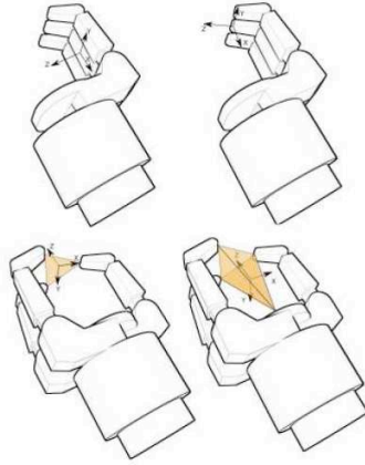
Figure 5: Task frames for the hook power (top-left), hook precision (top-right), precision (bottom-left) and cylindrical (bottom-right) preshapes [57].
