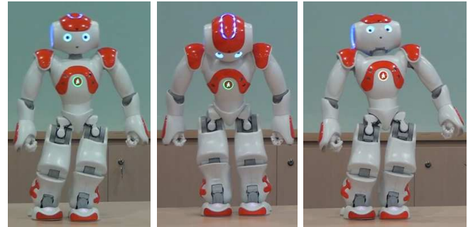
Fig. 1. A humanoid robot walking with three different styles. From left to right: relaxed, sad and proud.
