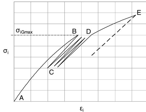
Fig. 6: Pre-failure material model for the UD Glass/Epoxy
