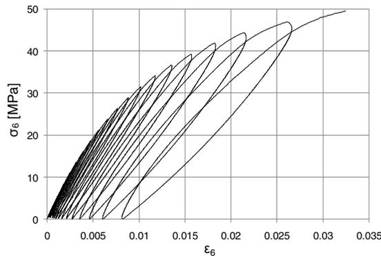
Fig. 1: Typical shear stress-strain cycles under static L-U-R
