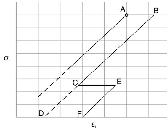
Fig. 7: Post-FF material model for the UD Glass/Epoxy
