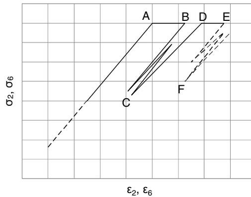
Fig. 8: Post-IFF material model for the UD Glass/Epoxy
