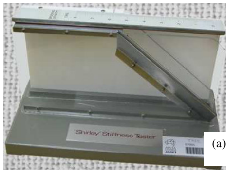
Fig. 6. (a) ASTM, Standard test method for bending stiffness of fabrics [48], (b) A representative bending test result [39]
