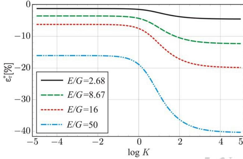
Figure 7. The effect of transverse shear deformation on critical buckling loads of geometrically perfect two-layer C-C composite column for various flexural-to-shear ratios  $E/G$  and different values of  $K$ ; where  $K$  [kN/cm<sup>2</sup>].
