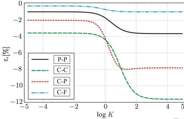
Figure 3. Comparison of the present critical buckling loads with those proposed by Xu and Wu [43] for  $E/G = 16$ , different types of boundary conditions and various values of  $K$ ; where  $K$  [kN/cm<sup>2</sup>].
