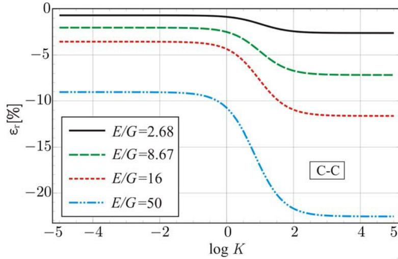
Figure 4. Comparison of the present critical buckling loads with those proposed by Xu and Wu [43] for C-C column case, different flexural-to-shear ratios,  $E/G$ , and various values of  $K$ ; where  $K$ [kN/cm<sup>2</sup>].
