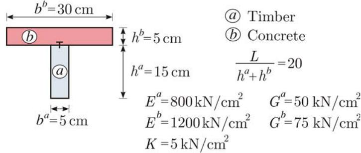
Figure 2. Geometrical and mechanical properties of timber-concrete column.
