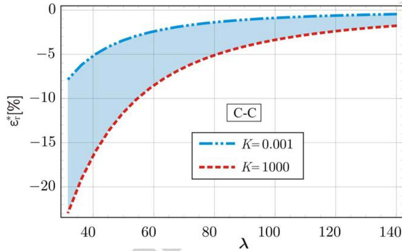
Figure 8. The effect of transverse shear deformation on critical buckling loads of geometrically perfect two-layer C-C timber ( $E/G = 16$ ) composite column for various column slenderness ratios  $\lambda$  and different values of  $K$ ; where  $K$  [ $\text{kN/cm}^2$ ].
