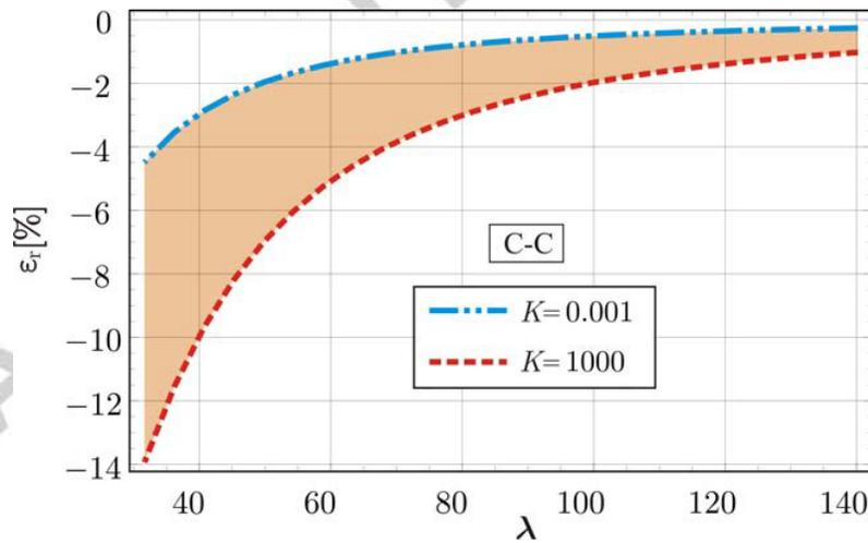
Figure 5. Comparison of the present critical buckling loads with those proposed by Xu and Wu [43] for C-C column case, different column slenderness ratios,  $\lambda$ , and various values of  $K$ ; where  $K$ [kN/cm<sup>2</sup>].
