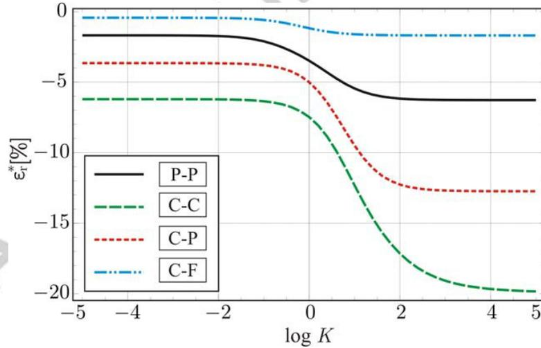
Figure 6. The effect of transverse shear deformation on critical buckling loads of geometrically perfect two-layer composite column with  $E/G = 16$  for various values of  $K$  and different types of boundary conditions; where  $K$  [kN/cm<sup>2</sup>].
