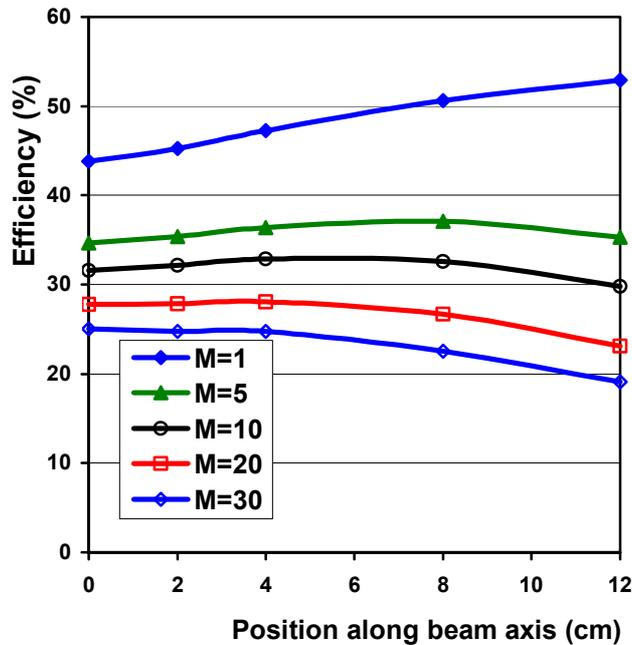
**Fig. 4.5:** Efficiency of tracked data as a function of position of the  $\gamma$ -ray source along the beam axis. The calculation has been done for  $E_\gamma = 1$  MeV.
