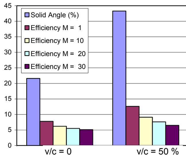
**Fig. 4.7:** Efficiency of the  $1\pi$  set-up for stopped and relativistic beams. Due to the kinematic focusing, the effective solid angle of the array increases by about a factor of two at  $v/c = 50\%$ .
