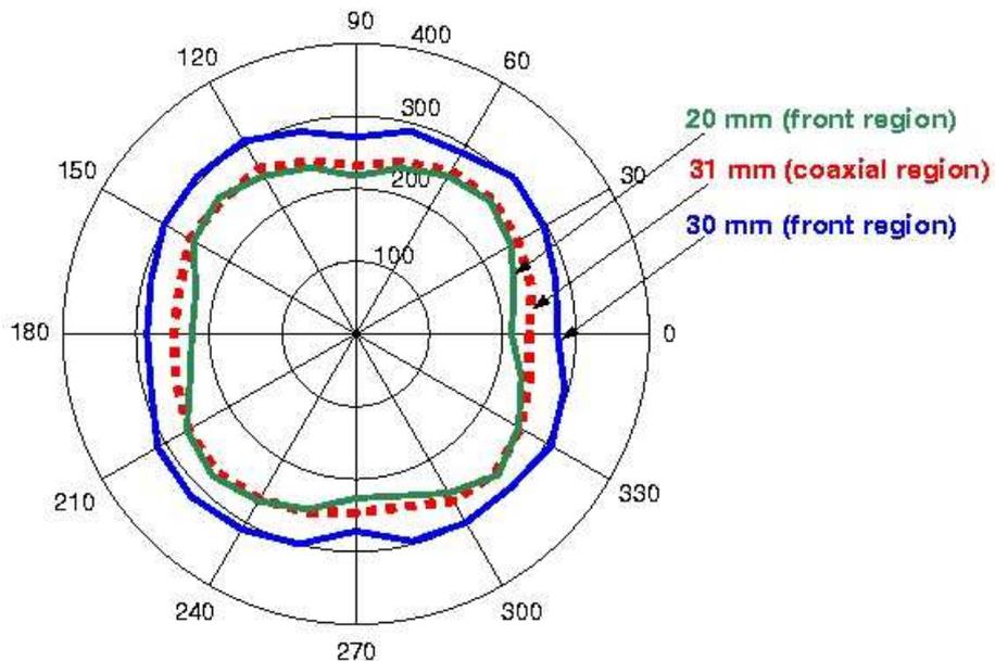
**Fig. 5.3:** Polar plot of the time-to-maximum (in ns) for pulses from  $60\text{ keV}$   $\gamma$  rays emitted from a  $^{241}\text{Am}$  source measured with a Ge detector. The angles  $0^\circ$  and  $90^\circ$  correspond to the  $\langle 100 \rangle$  and  $\langle 010 \rangle$  crystallographic directions, respectively.
