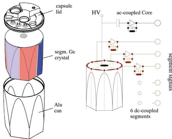
**Fig. 2.6:** *The encapsulated six-fold segmented MINIBALL detector.*
