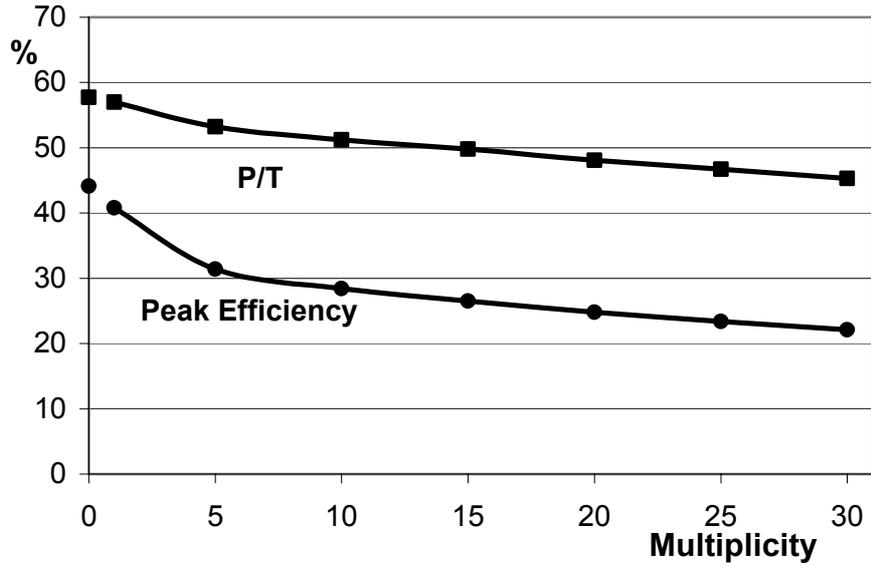
**Fig. 4.4:** Efficiency and P/T of AGATA as a function of multiplicity for cascades of 1 MeV transitions. The values at  $M=0$  are the response of the array, obtained summing all interaction points. The other, tracking, results depend on the assumed position resolution and will improve following the development of the reconstruction algorithms.
