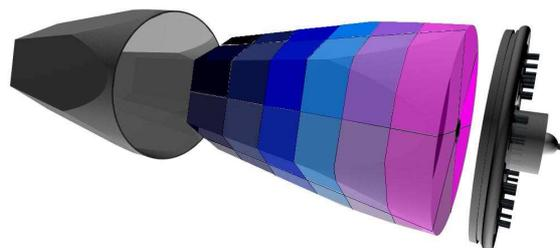
**Fig. 4.9:** The 36-fold segmented, encapsulated Ge detector
