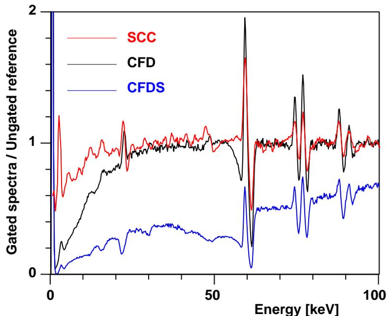
**Fig. 5.4:** Measured efficiency of the SCC discriminator (red line) compared to that of an analogue Constant Fraction Discriminator (Canberra model 1326A) for two different parameter settings optimised for low threshold (black line) and good timing (blue line), respectively.
