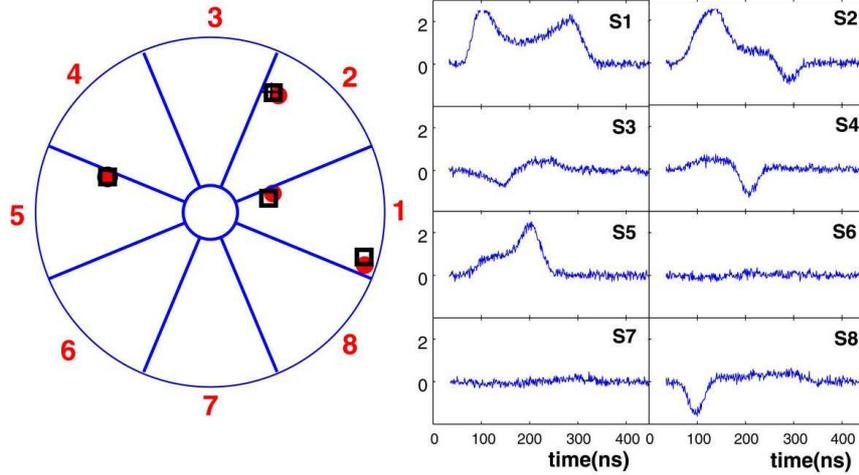
**Fig. 5.6:** Cross section of a 8-fold segmented coaxial Ge detector with simulated interaction points (dots) and derived positions (open squares). The interaction points are at different depths in the detector. The left panel shows the simulated current pulse shapes, with added noise, as seen in the eight segments.
