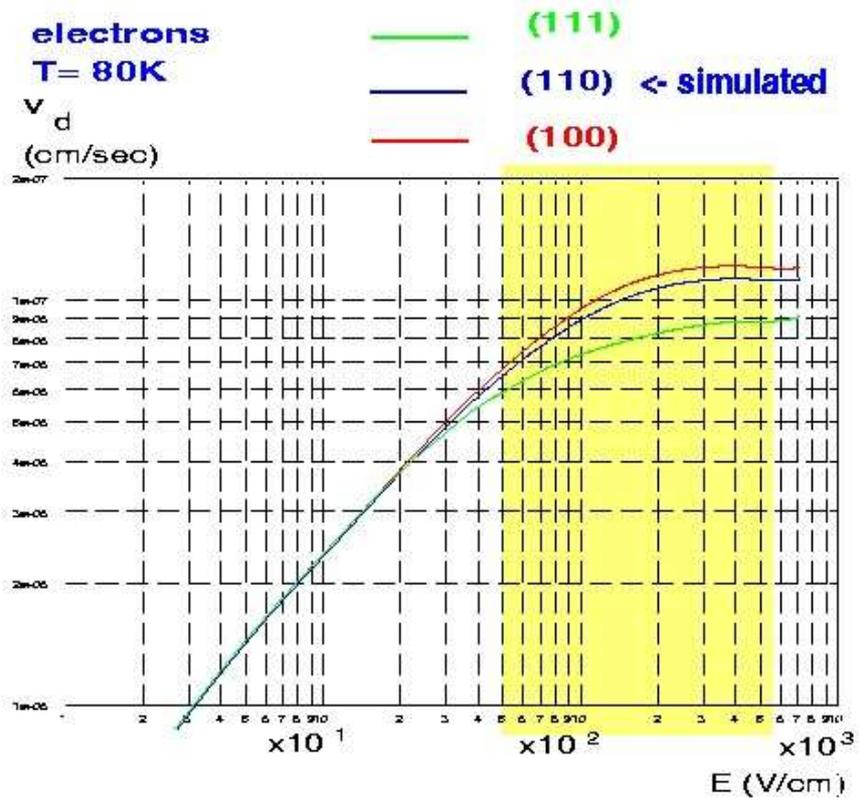
**Fig. 5.2:** The experimental drift velocities of electrons in a Ge crystal along the  $\langle 111 \rangle$  and  $\langle 100 \rangle$  directions at a temperature of  $T = 80\text{ K}$  and the simulated drift velocity for a field oriented along the  $\langle 110 \rangle$  direction.
