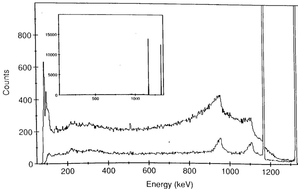
**Fig. 2.2:** Unsuppressed and suppressed  $^{60}\text{Co}$  spectra obtained with a Eurogam Phase 1 ESS. The y-axis has been scaled to show the details of the background. The insert showing the full photopeak intensity relative to the background indicates the overall quality of the spectrum.
