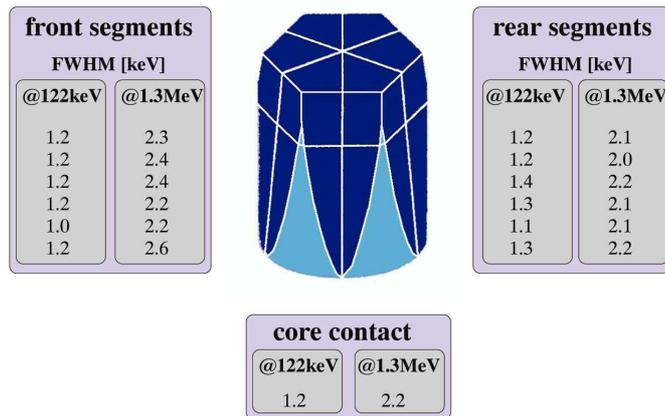
**Fig. 2.9:** *The 12-fold segmented, encapsulated Ge detector.*
