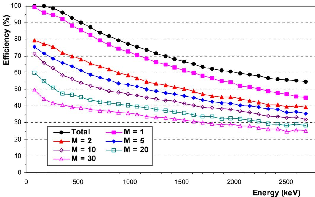
Fig. 3.15: Efficiency of an ideal shell as a function of transition energy and multiplicity.
