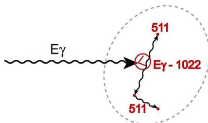
**Fig. 3.9:** Pair production interaction. The electron and positron, which release their kinetic energy within a few mm of the interaction point, are seen as one point. The annihilation photons have their own absorption history and generate two  $\gamma$  ray tracks originating from the interaction point.
