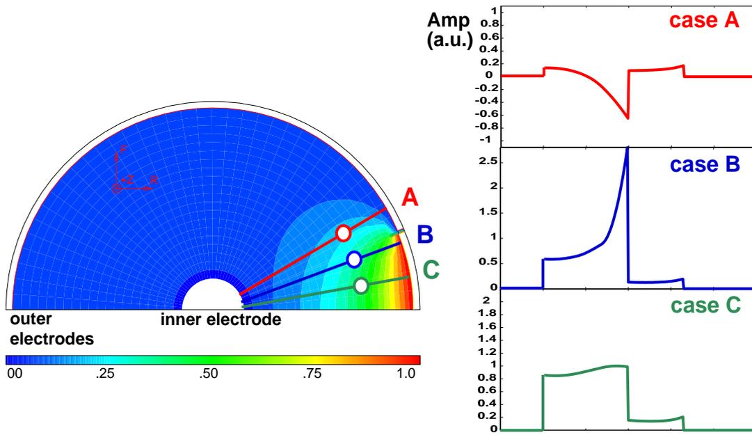
**Fig. 3.3:** *Weighting potential of a segment in a coaxial detector with three examples of interactions occurring at the same radius, but at different azimuthal angles (left), and the corresponding induced current signals (right).*
