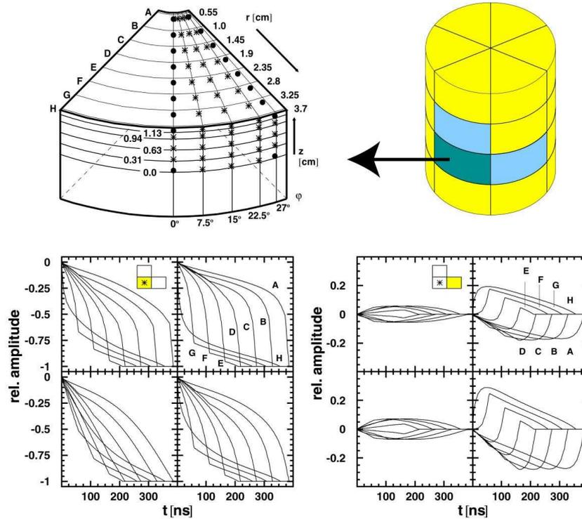
**Fig. 5.1:** Calculated pulse shapes for the coaxial part of a closed-end Ge detector. The real charge pulses shown in the four graphs of the lower left panel are due to interactions at different radii, azimuthal angles, and longitudinal positions in the upper right quarter of the selected segment (indicated by dots). The corresponding transient mirror charge pulses in the neighbouring horizontal segment are shown in the left panel.
