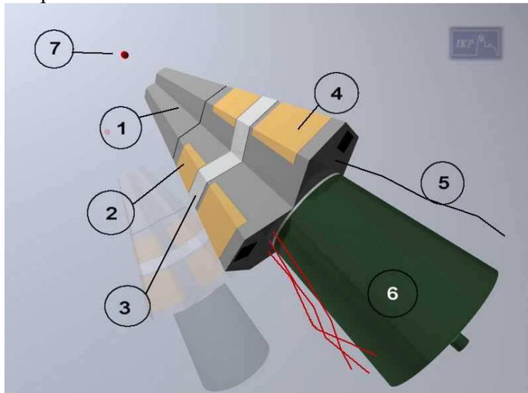
**Fig. 4.8:** The  $\gamma$ -ray tracking module: ① Cryostat end cap containing the 36-fold segmented Ge detectors, ② pre-amplifier section, ③ support frame, ④ digital front-end electronics, ⑤ fibre-optic channel readout, ⑥ LN2 dewar, ⑦ radiation source.
