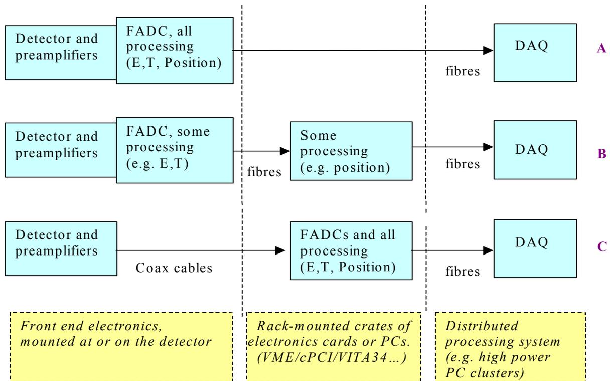
**Fig. 6.1:** Various options for distribution of processing.
