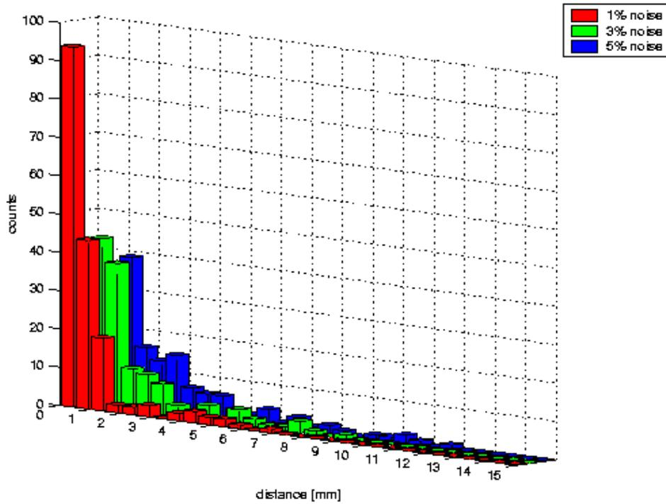
**Fig. 5.7:** Position resolution of the WPC identification system in three dimensions for three different noise levels.
