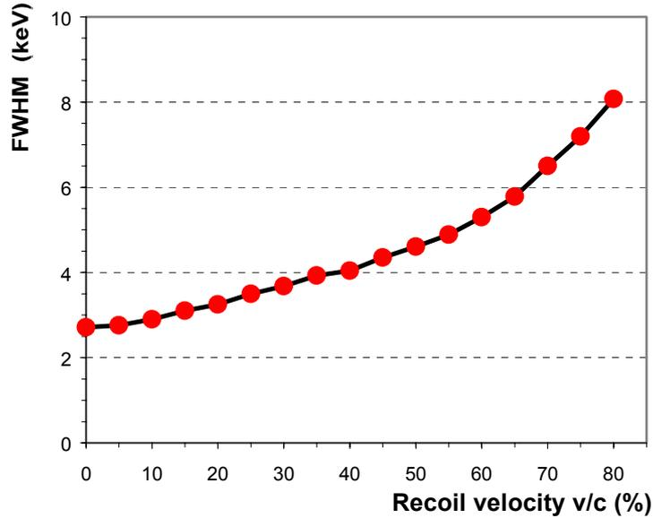
**Fig. 3.17:** Energy resolution of reconstructed and Doppler corrected 1.33 MeV transitions as a function of the velocity of the emitting source. Direction and velocity of the source are supposed to be perfectly known.
