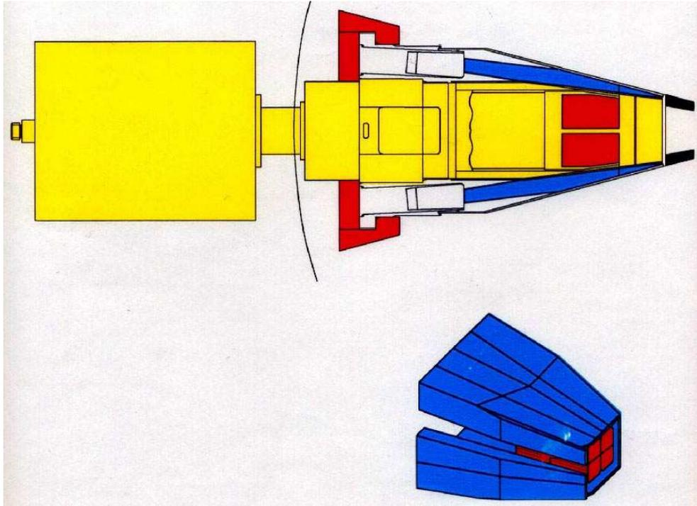
**Fig. 2.1:** A schematic diagram of a modern escape suppressed spectrometer. The figure shows a Clover Ge detector of the Euroball array inside its BGO escape suppression shield comprising of 16 individual crystals.
