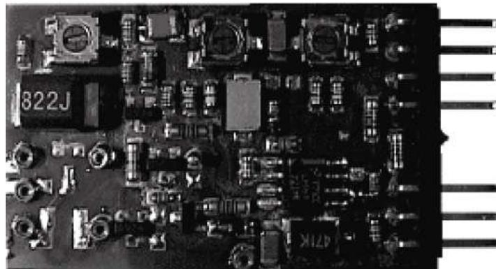
**Fig. 2.8:** *The SMD-Preamplifier. Gain: 175mV/MeV;
