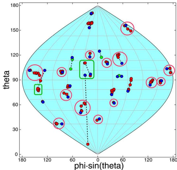
**Fig. 3.12:** “World map” representation of an  $E_\gamma = 1.0$  MeV,  $M_\gamma = 30$  event detected in the ideal germanium shell and reconstructed with the “cluster-tracking” algorithm. Correctly reconstructed transitions are encircled and represent about two thirds of all  $\gamma$  rays in the event; the two rectangles represent badly reconstructed background events. About 75 % of the original transition is reconstructed correctly.
