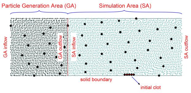
Figure 11: Particle Generation Area (GA) and Simulation Area (SA)
