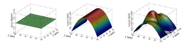
Figure 2: Poiseuille flow simulated with DPD: uniform density distribution (left) and parabolic velocity distribution (middle). The change in the velocity profile as the result of the clot formation (right).
