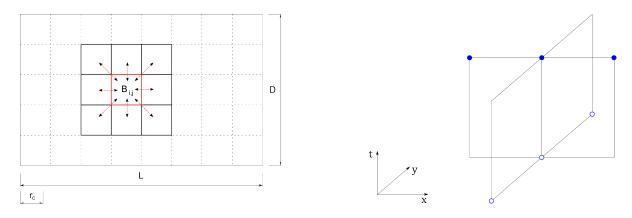
Figure 10: Left: a scheme of the optimization technique for the calculation of inter-particle forces. Right: alternating direction implicit (ADI) method stencil for the first half-step - implicit in the x and explicit in the y direction.
