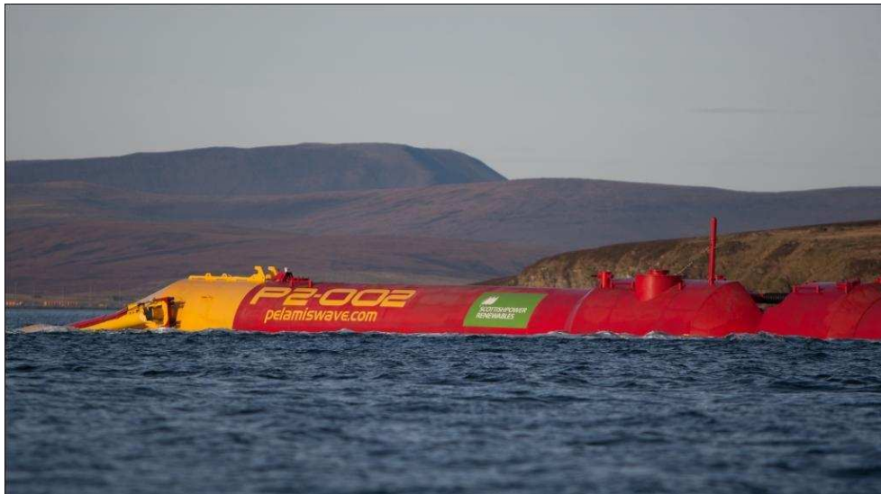
FIGURE 1. Pelamis Wave Power Device, picture from http://www.pelamiswave.com
