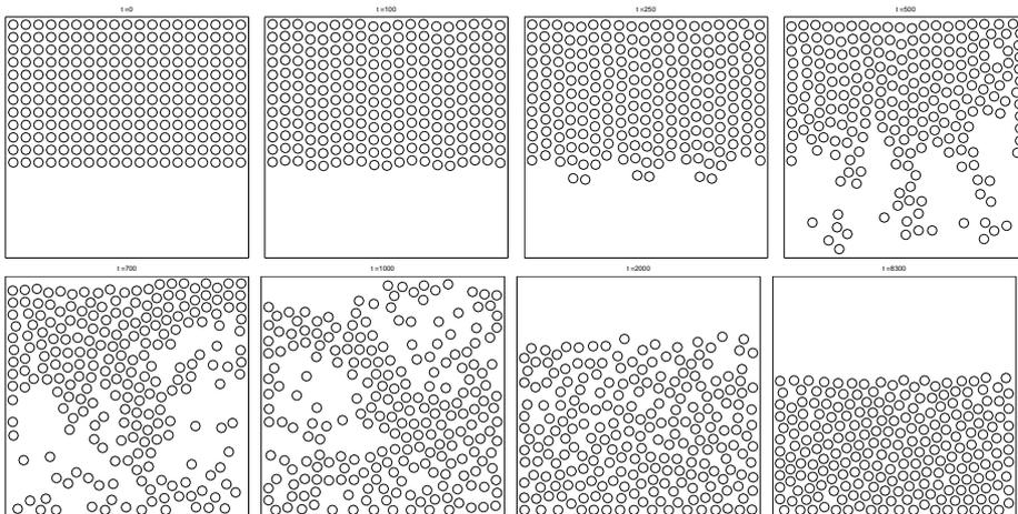
Figure 9: Sedimentation of 228 particles: configurations at different time steps.
