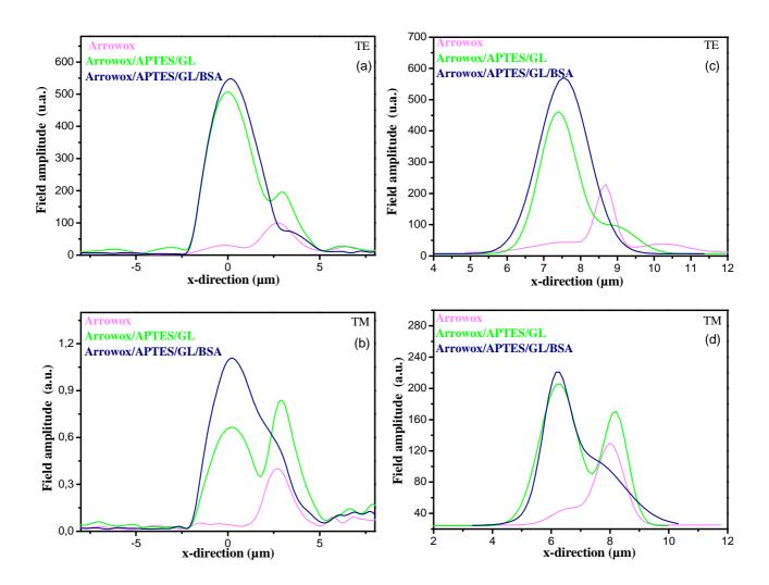
Fig. 4. Near-field profiles: BPM simulated for TE (a) and for TM (b) and experimental for TE (c) and for TM (d).
