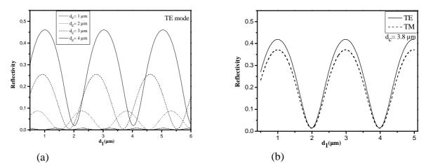
Fig. 2. Calculated reflectivity as a function of  $d_1$  (a) for four different thicknesses  $d_c$  in ARROW structure for the TE mode and (b) for  $d_c = 3.8 \,\mu\text{m}$  for both TE and TM modes, with refractive index values  $n_c = 1.356$ ,  $n_1 = 1.396$ ,  $n_2 = 1.350$  and working wavelength  $\lambda = 1.55 \,\mu\text{m}$ .
