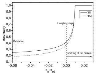
Fig. 3. Calculated reflectivity as a function of the refractive index variation of the core layer after each step (functionalization and BSA grafting), with constant values of  $n_1$  and  $n_2$  for TE and TM modes, working wavelength  $\lambda = 1.55 \ \mu m$ ,  $d_c = 3.8 \ \mu m$  and  $d_1 = 1.4 \ \mu m$ .
