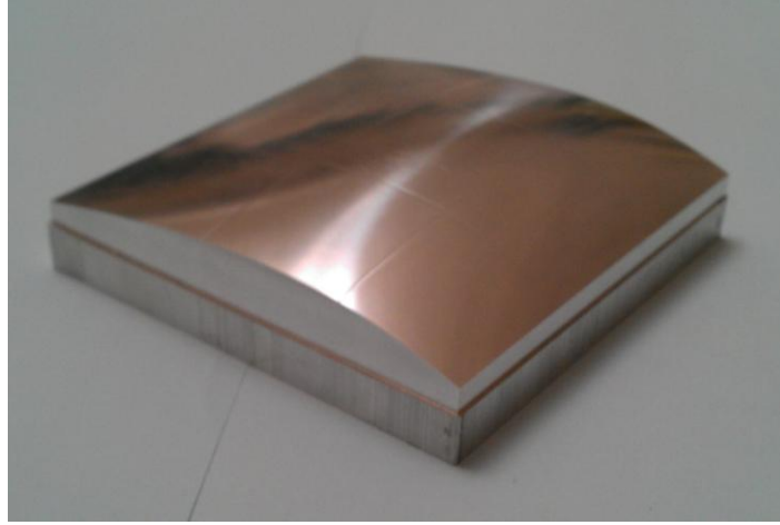
Figure 1: Part made of aluminum alloy and machined with an HSM.
