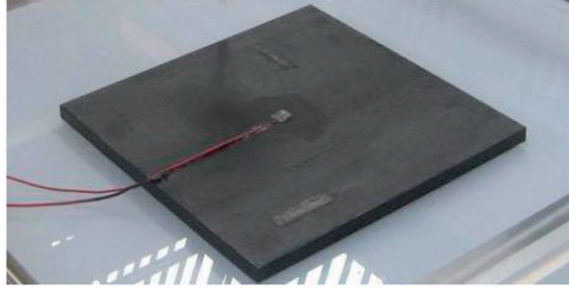
Figure 14. Steel mock-up created with two rectangular defects and one anodic protection.
