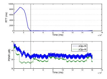
Fig. 3. Measured RTT and PSNR ( $RTT_i = 20$ ms, bandwidth: 2.5Mbps).
