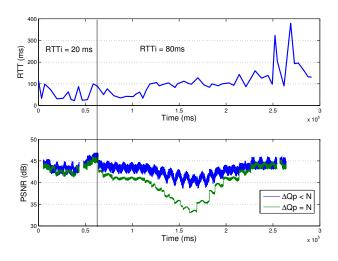
Fig. 5. Measured RTT and PSNR  $(RTT_i = 20ms \text{ and } 80ms, \text{ bandwidth: 5Mbps}).$
