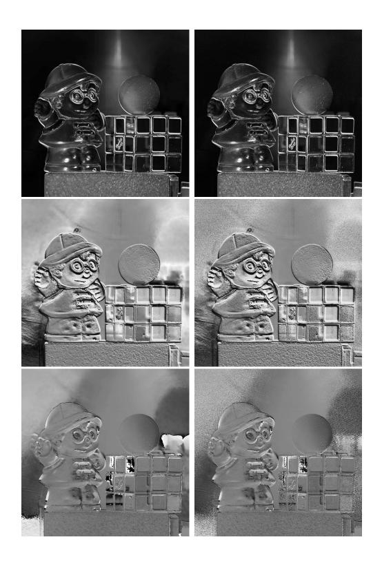
Fig. 4. Degree of polarization (first line), ellipticity (second line) and orientation (third line) of the Stokes vectors estimated with the proposed approach (left), and by using the pseudo-inverse (right).
