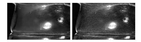
Fig. 5. Degree of polarization of the Stokes vectors estimated with the proposed approach (left) and by using the pseudo-inverse (right). The zoom in on the foot of the figurine reveals the denoising efficiency of the proposed approach.
