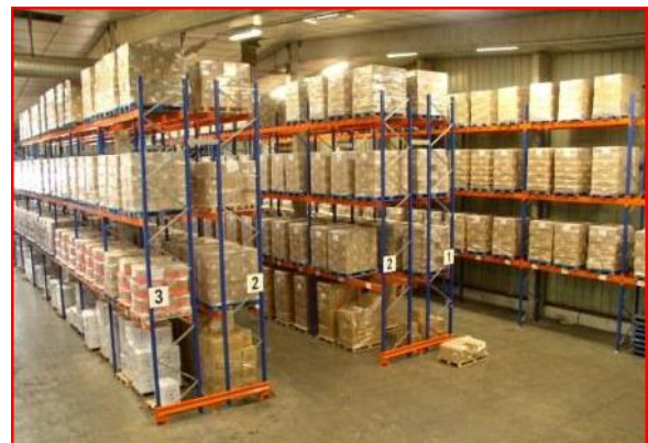
Figure 1: Stockage en rack
