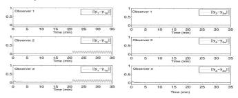
Fig. 5. Residual vector with a fault in the first sensor.
