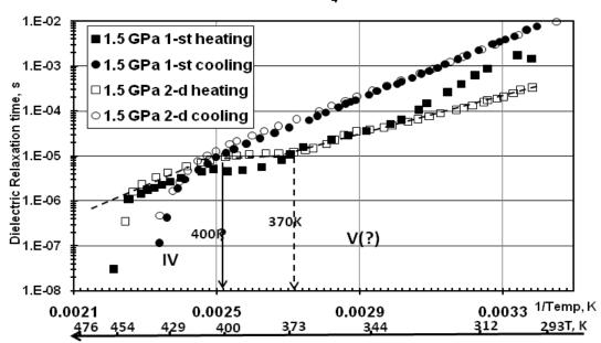
**Figure 5** Electrical conductivity  $\sigma$  and dielectric relaxation time  $\tau$  at 1.5 GPa: phase I and VI are superprotonic, phases
