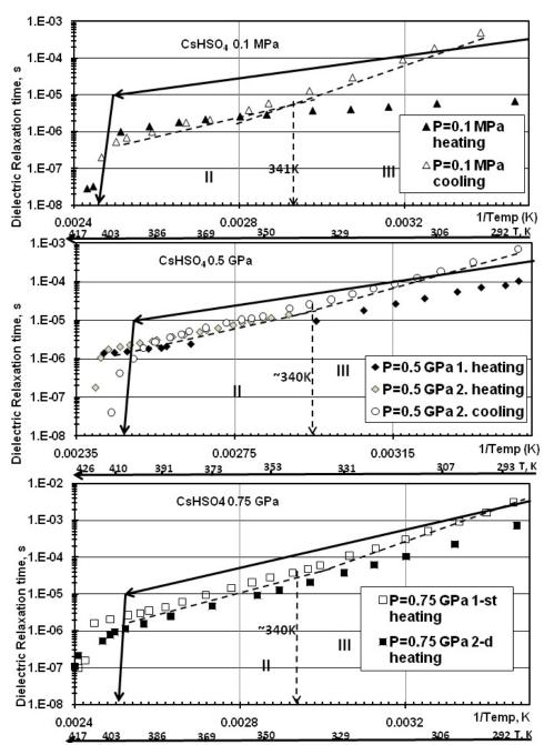
**Figure 2** Dielectric relaxation time in CsHSO<sub>4</sub> at 0.1 MPa, 0.5 and 0.75 GPa. Solid arrows indicate the drop of the mean residence time  $\tau_H$  of spin-lattice relaxation [19].
