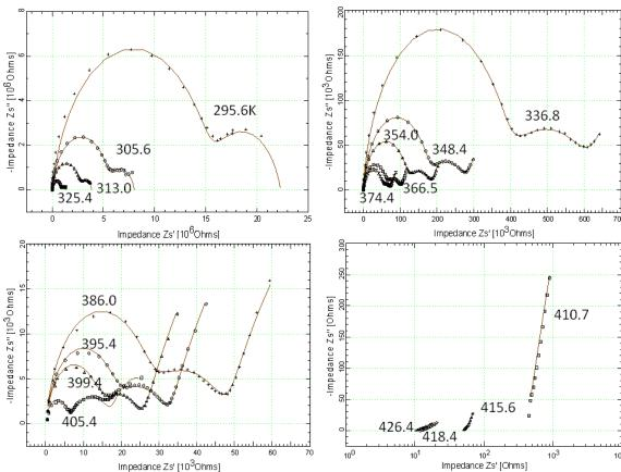
Figure 3 Evolution of impedance spectra at P=0.1 MPa. The Phase transition II=> I corresponds to the abrupt change of impedance spectra (right lower panel). The left arc in the Argand plots is the bulk impedance; the small intermediate arc is probably the grain boundary phase impedance. The right shoulder of the spectra is Wagner impedance branch. The parameter p from Eq 1 varies from 0.89 at 295.6 K to 0.80 at 405.4 K.
