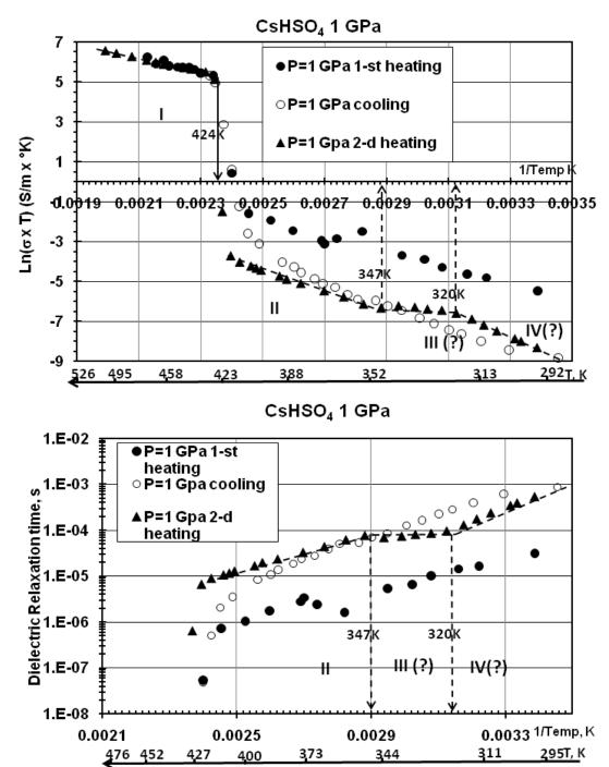
**Figure 4** Electrical conductivity  $\sigma$  and dielectric relaxation time  $\tau$  at 1 GPa: phase I is superprotonic, phases II-IV are
