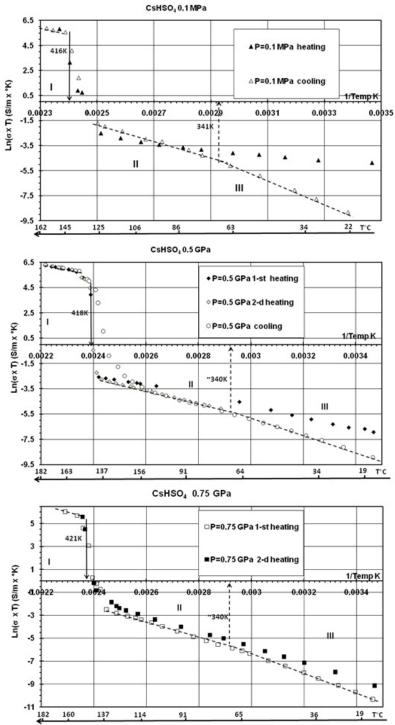
Figure 1 Electric conductivity in  $CsHSO_4$  at 0.1 MPa, 0.5 and 0.75 GPa.
