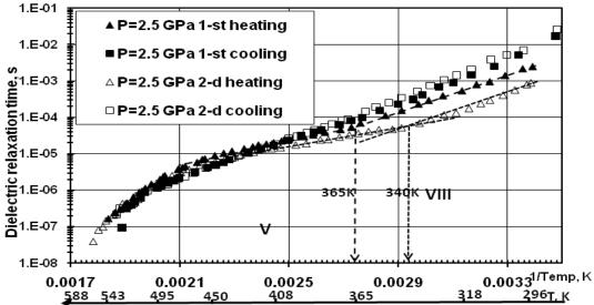
**Figure 7** Electrical conductivity  $\sigma$  and dielectric relaxation time  $\tau$  at 2.5 GPa, phases V and VIII are probablynot ferroelastic, small knick in slope is observed during cooling cycle.
