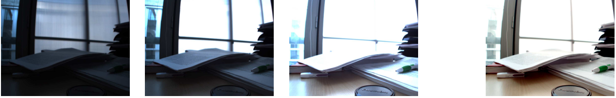
Figure 5: Images of a test scene under different exposure times (columns 1 to 3). Linearly tone-mapped photoquantity of the test scene obtained with our method (column 4).
