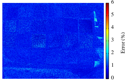
Figure 8: Relative error resulting from ignoring noise during photoquantity computation (same scene as Fig. 6).
