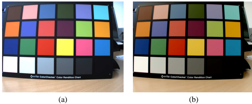
Figure 6: Study of the linearization and colour-correction accuracy of the method: uncorrected LDR image (a) and corrected HDR image (b).
