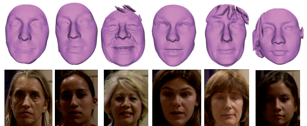
Fig. 17: Different female 3D faces misclassified by our approach. The first row shows 3D data, the second shows the corresponding texture of 3D data.
