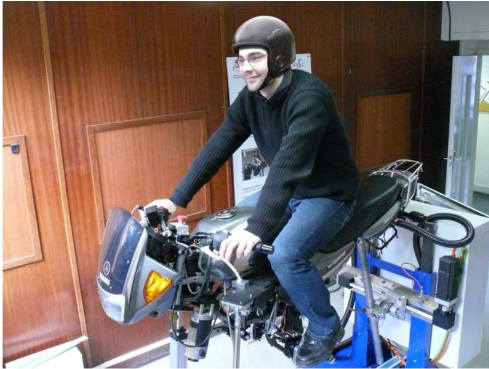
Fig. 1. SIMACOM's Riding Simulator Platform (INRETS-UEVE)
