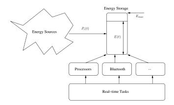
Figure 1. Energy Harvesting Embedded System Model
