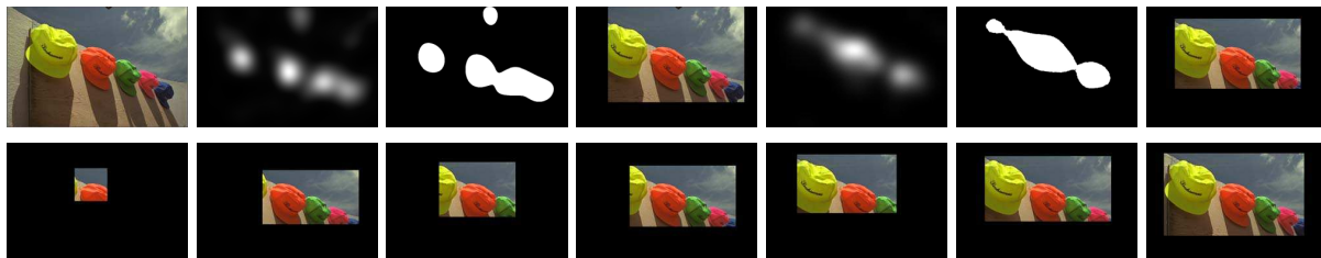
FIGURE 5: Top row, static re-purposing (from left to right): original image, ground-truth heat-map, binarized ground-truth heat-map, cropped image from ground-truth GT , heat-map from simulation, binarized heat-map from simulation, cropping from simulation S . Bottom row : dynamic re-purposing from simulation SF_t , frames 1,50,100,150,200,250 and 300.
