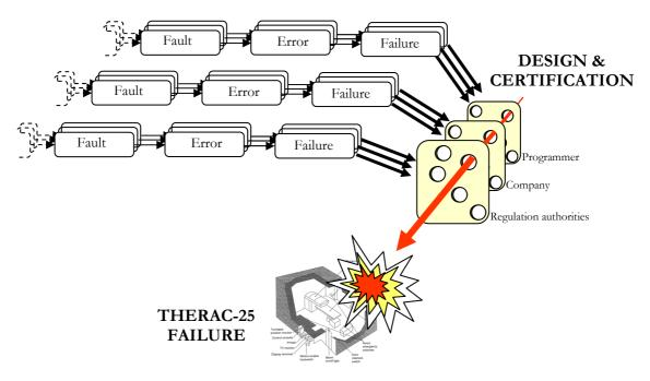
Figure 4: Faults, errors and failures generating impairments in some of THERAC-25 systems' layers.
