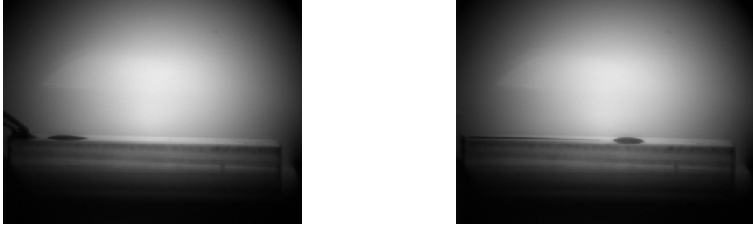
Fig. 3. Side view of the water droplet actuated by the ethanol droplet at two different times. The water droplet moves from left to right.
