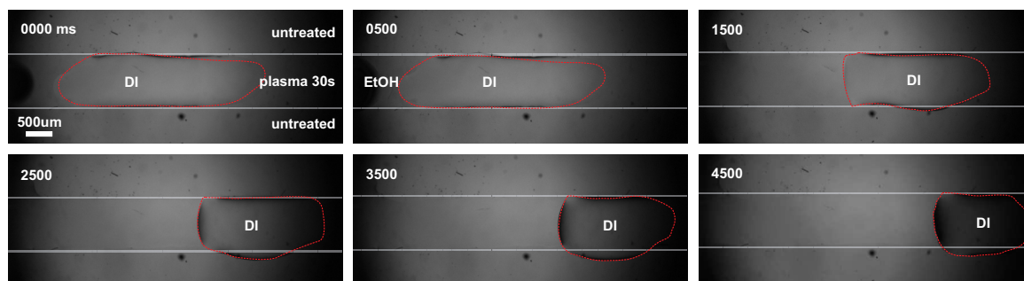
Fig. 2. Picture sequence showing from above the actuation of the water droplet by an ethanol droplet on an hydrophilic highway.
