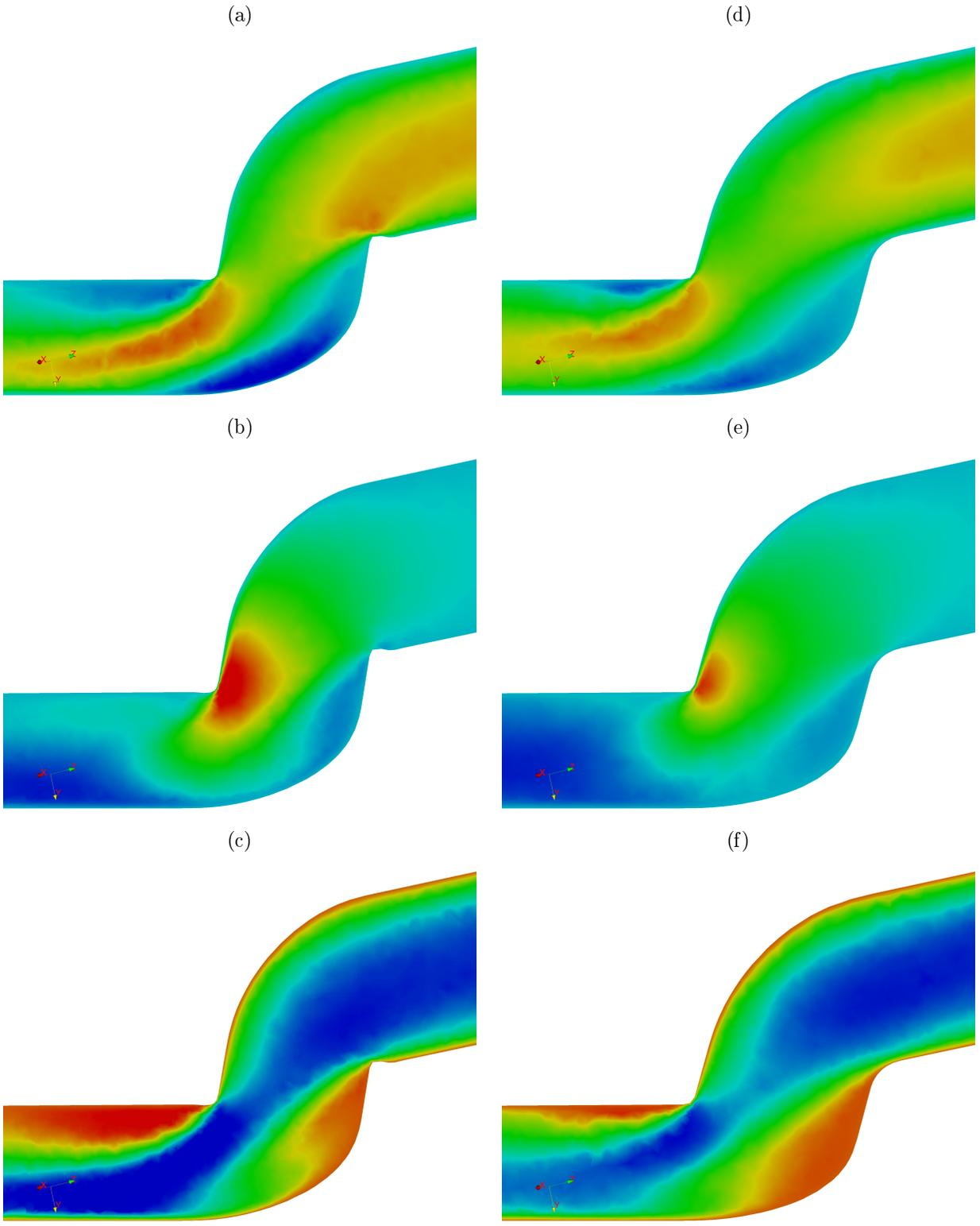
Figure 5: Velocity fields:  $x$ -components (a,d),  $y$ -components (b,e), and  $z$ -components (c,f). The first column corresponds to the worst observed scenario; the second column shows the optimized fields.
