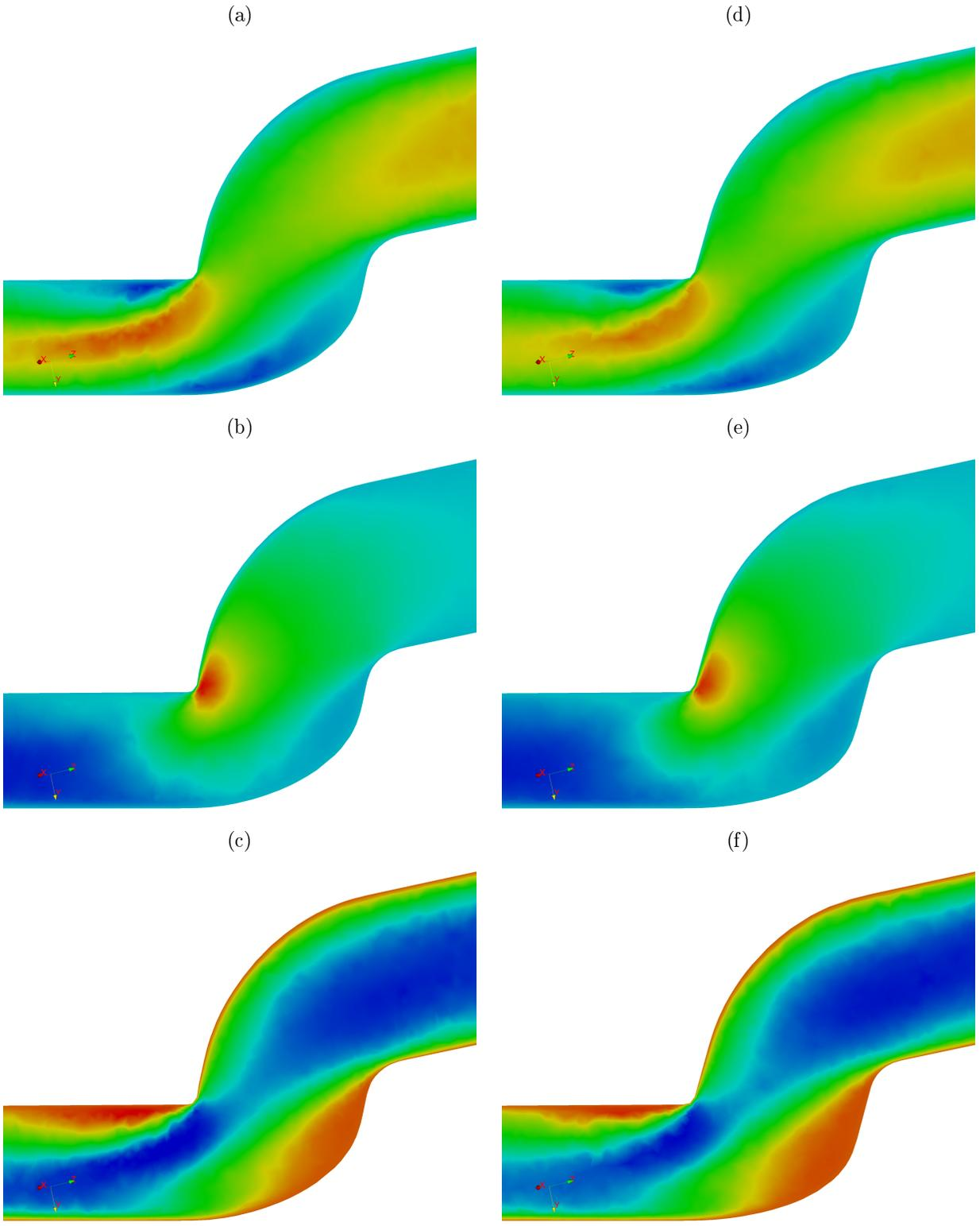
Figure 6: The components of the velocity field of a flow:  $x$ -direction (a,d),  $y$ -direction (b,e), and  $z$ -direction (c,f). The first column corresponds to the result in [31]; the second column is our result which is the replica of the second column in Fig. 5.
