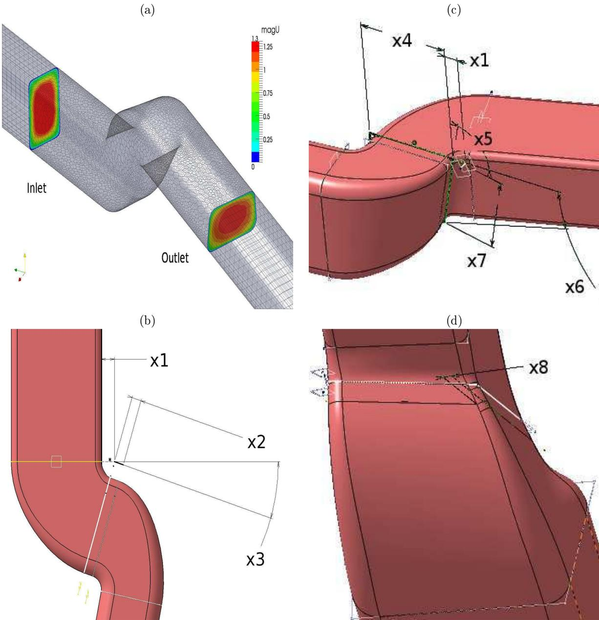
Figure 1: Optimization criterion is the difference between the average (normalized) pressure field at the inlet and outlet (a). The optimization parameters are  $x_1$ - $x_3$  (b),  $x_1$ ,  $x_4$ - $x_7$  (c), and  $x_8$  (d).
