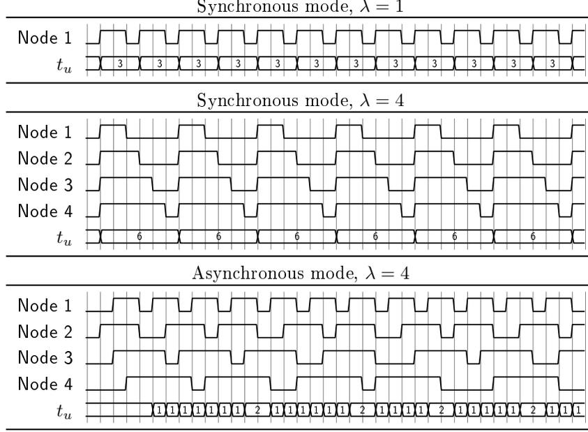
Figure 12: Advantages of the asynchronous node access. In the synchronous case with  $\lambda = 1$ , WCT = 3. Adding three slower Nodes 2–4 allows to have four simultaneous evaluations, but the wall clock time will be determined by the worst node. However, the asynchronous access reduces the  $t_u$  values to  $t_b$  for the majority of expensive function evaluations.
