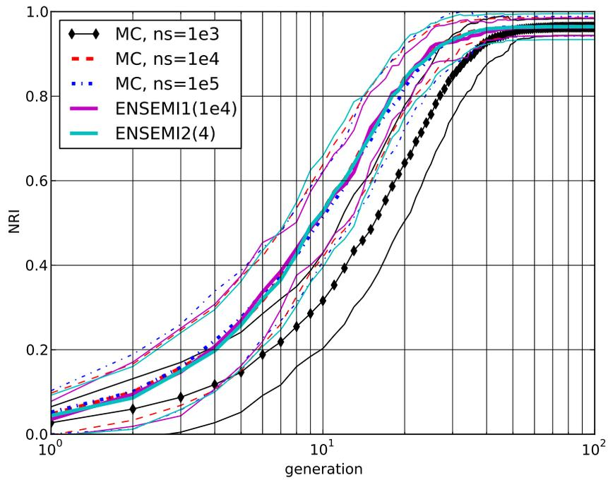
Figure 22: Solution of the "ranklapprox9d" problem by using the synchronous algorithm with the  $EI^{0.4}$  criterion and various integration methods applied to estimate the multi-point EI criterion. The ENSEMIx rules outperform the MC method with  $ns = 10^3$ , and yield similar results when  $ns = 10^4, 10^5$ .
