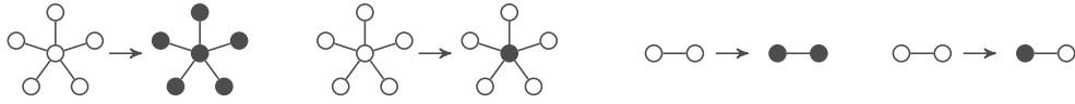
Figure 1: Scopes of local computation. Nodes in the scope of preconditions are filled in white, while nodes affected by the actions are filled in black (reproduced from Casteigts et al. [CCF12]).
