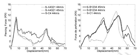
Figure 11. Comparisons (a) between graded core S-A4321 and homogeneous core S-C4 and (b) S-B1234 with S-C1.
