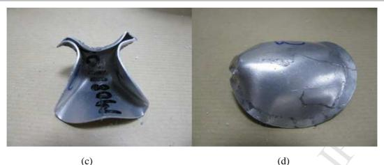
Figure 9 Post-mortem observations of the top and bottom skins for S-A4321 (a),(b) and S-B1234 (c) and (d).
