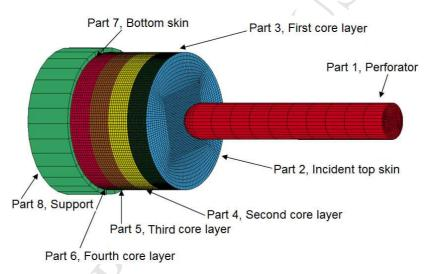
Figure 13 Numerical model for the perforation of a sandwich sample
