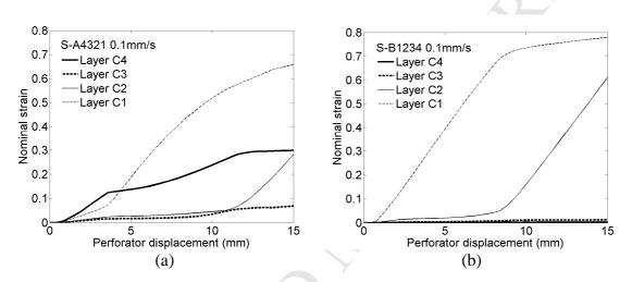
Figure 18 Nominal strain evolution for S-A4321(a) and S-B1234 (b) quasi-static loading.
