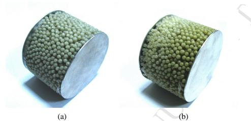
Figure 2 The Photograph of sandwich sample with homogeneous core (a) and graded core (b)
