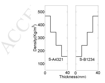
Figure 1: The graded profile of the S-A4321 and S-B1234 sandwich plates
