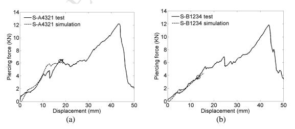
Figure 18 Comparisons between tests and simulations for graded core sandwich plates S-S-A4321 (a) and S-B1234 (b) under quasi-static loading.
