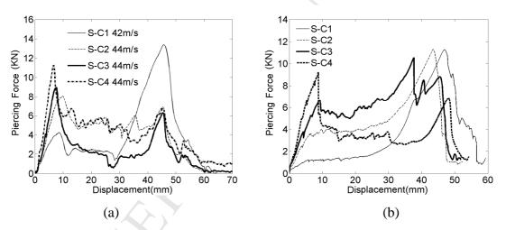
Figure 6: Piercing force vs displacement curves for homogenous sandwich under impact (a) and static (b) loadings
