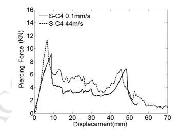
Figure 7 Comparison between quasi-static and impact perforating force for sandwich S-C4.
