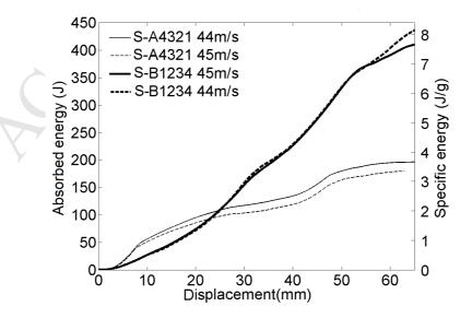
Figure 12. Energy absorption during piercing process.
