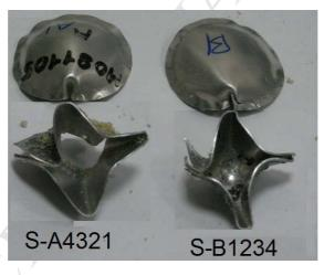
Figure 10 Post mortem photos sandwichs under quasi-static perforation
