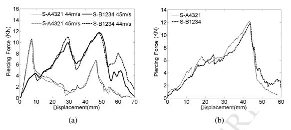
Figure 8. Piercing curves of sandwich with graded cores at 45m/s (a) and at quasi-static loading (b)
