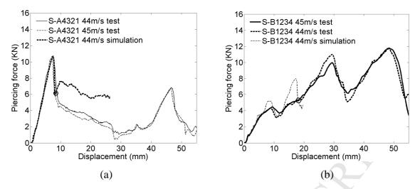
Figure 15 Comparisons between tests and simulations for graded core sandwich plates S-S-A4321 (a) and S-B1234 (b) under impact loading.
