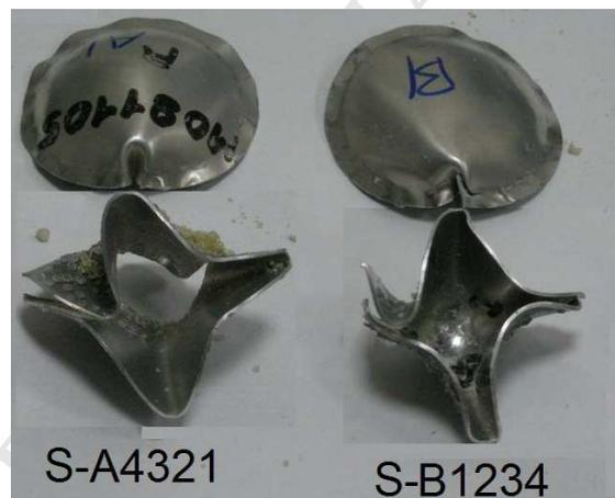
Figure 10 Post mortem photos sandwiches under quasi-static perforation
