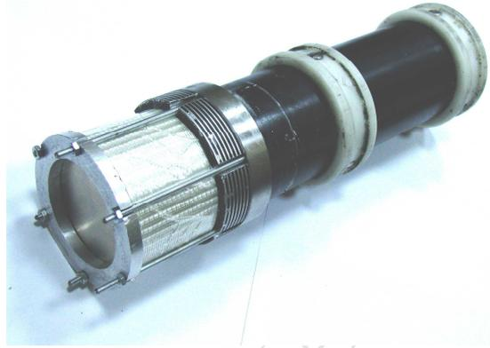
Figure 4. Photograph of the projectile/specimen system
