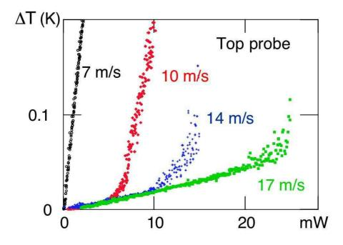
Figure 9: Temperature of the top probe as a function of the applied power in mW, for different flow velocities (T=1.80 K, liquid height  $\approx 3.5$  mm). The temperature is controlled by the Kapitza resistance between the aluminum plate and the deposited liquid film below a critical heat flux, and by exchange with the turbulent vapor above. Like the mist density, the critical heat flux, which corresponds to full vaporization of the deposited liquid flow, increases with the vapor velocity.
