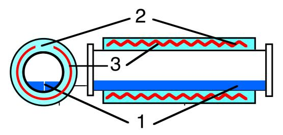
Figure 4: Characterization of the global heat transfer using the Kapitza box. The temperature difference between pressurized (2) and saturated (1) helium is measured as a function of the power  $W_K$  applied to the heater (3).
